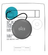
Applied to the meter, the sensor reads the blinks and transmits them to the DiCE SMART device.
